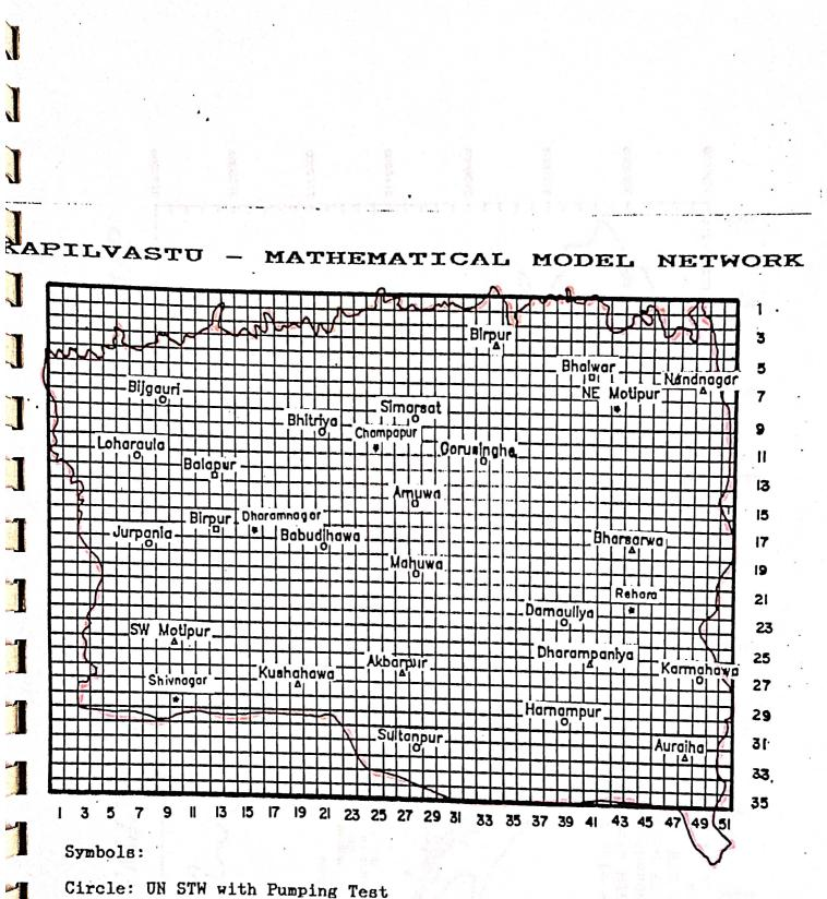
Circle: UN STW with Pumping Test Triangle: UN STW without Pumping Test Square: ADBN STW only Pumping Test Star: USAID STW with Pumping Test
